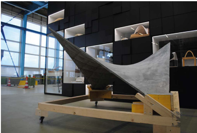
Fig. 13. This is the second prototype constructed at ETH Zurich for the HiLo project. It was used to demonstrate low construction tolerances.
