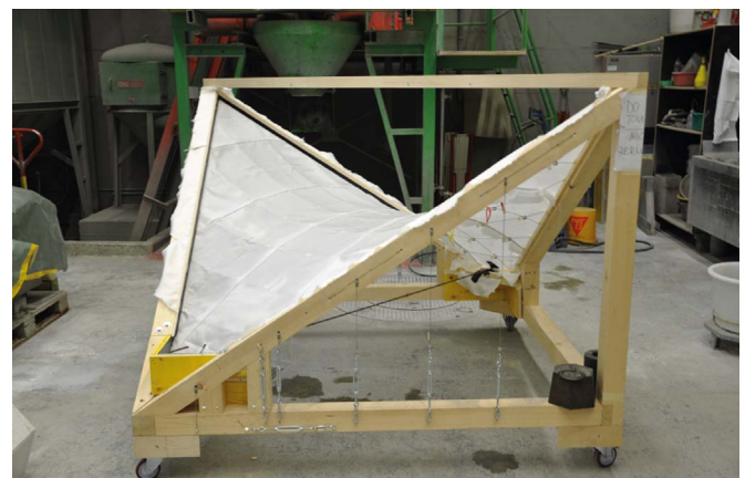
Fig. 12. The second prototype showing the timber frame and the prestressed cable net.
