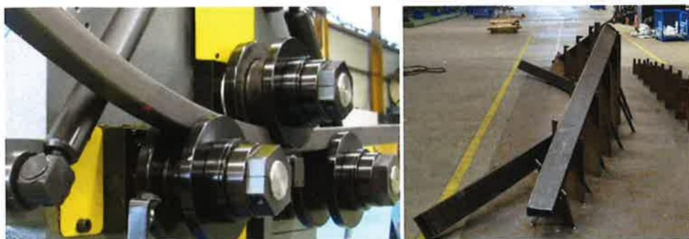
Fig. 13 Typical bending process (left) and double-curvature steel member by Kersten Europe (right)
