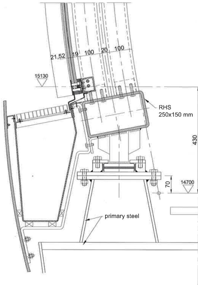
Fig. 9. Section through edge beam showing typical bearing detail (Knippers Helbig)
