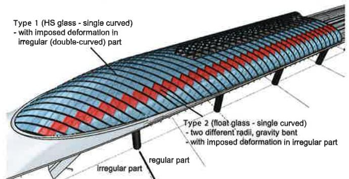
Fig. 5. Roof geometry consisting of irregular (double-curvature) and regular (generic) part, and locations of different glass types (Knippers Helbig)
