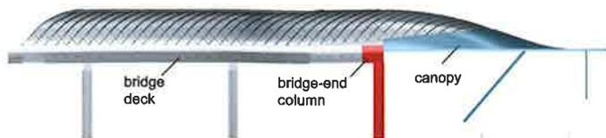
Fig. 6: Roof supported by three different structures (Knippers Helbig)
