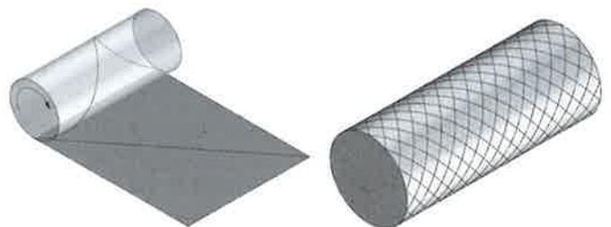
Fig. 10. General principle behind glass and steel geometry (Knippers Helbig)
