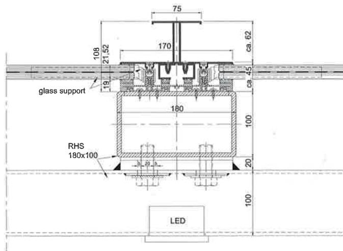
Fig. 7. Section through bolted connection (Knippers Helbig)
